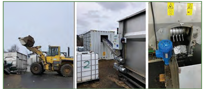
Figure 7. Watered silage loaded into a feeder to be pressed by a mechanical screw press
