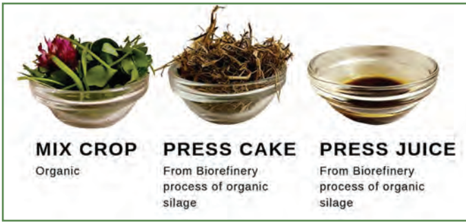
Figure 4 a. Organic or sustainably produced grass-clover silage as a green biorefinery input feedstock b. green biorefinery press cake and c. green biorefinery protein juice processed into high value organic protein products and amino concentrate feeds for pigs and chickens.
